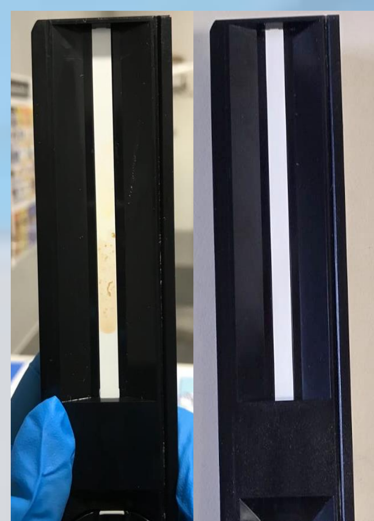
Figure 5: dirty vs clean calibration bar
